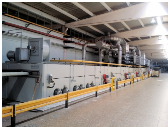
The energy efficient KMA ULTRAVENT system reduces the energy costs of the stenter frame machine.
