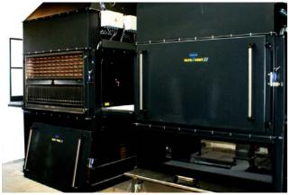
Pict.: ULTRAVENT  $^{\otimes}$  air filter with demister, electrostatic precipitator and heat exchanger (from the bottom upwards). The automatic filter cleaning system is placed between the electrostatic filter and heat exchanger module.
