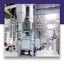
This drips off the collection plates and is collected in a recuperation tank. The oil separated here can often be reused. The second type forms a greasy, oily or encrusted deposit on the filter surface. Unsuitable filter types can quickly clog and become ineffective, leading to excessive costs associated with filter replacement and disposal. However, electrostatic precipitators never obstruct the air flow through the exhaust system.
