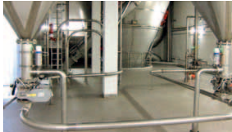
AAIRMAXX ® ESP filters with discharge airlocks and tubes for transport of discharged powder
