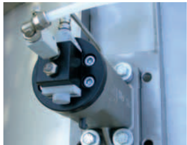
Pneumatic impactor on the outside of the filter tube
